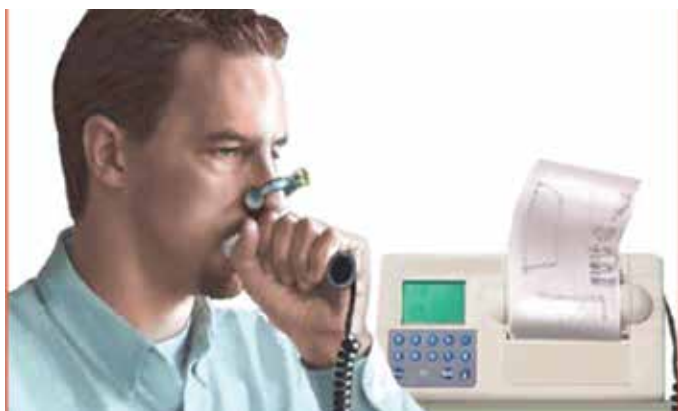
Fig. 1: Simple desktop spirometer
